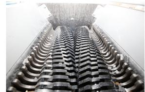
Stage 2: fine shredding using a two-shaft system.
