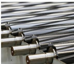
The induction-hardened, solid steel cutting rollers can easily cope with staples and paper clips and guarantee durability.
