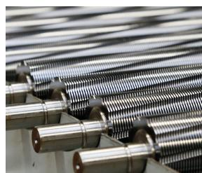
The induction-hardened, solid steel cutting rollers guarantee durability.
