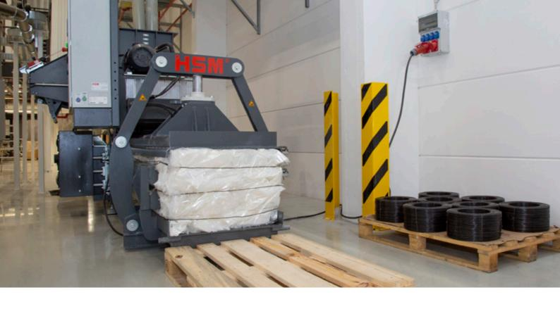
The HSM VK 2306 is comparable with the HSM VK 1206, but features a higher pressing power. It produces highly compressed PET bales which are marketable immediately – no additional compression required.
