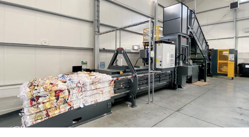
For professional disposal management or larger industrial applications – with high throughput rates of up to approx.  $442 \text{ m}^3/\text{h}$ .
