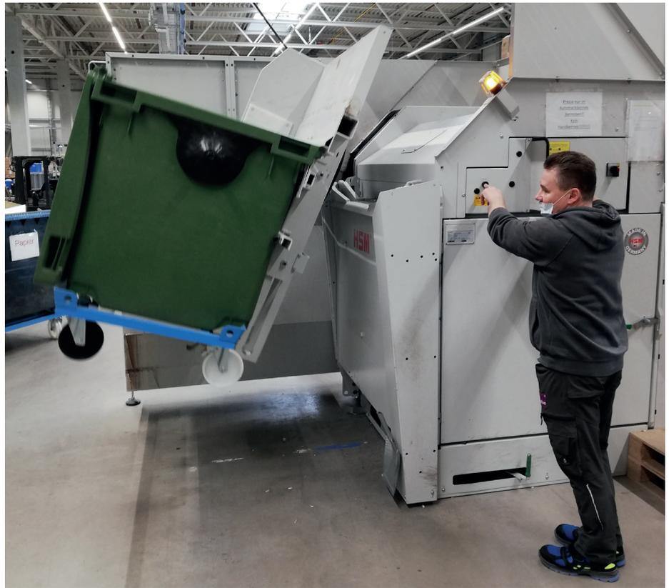
now conveyed in a tugger train, they are efficiently integrated into Alber's Intralogistics: a tugger train can pull four waste bins to the baling press at the same time. The result is a process which is four times as fast whilst also saving unnecessary trips. According to Alber, the whole concept works only because the HSM press fulfills the requirements so well.
