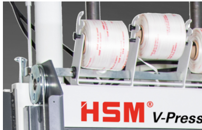
Manual bale strapping with continuous polyester tape
