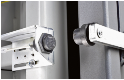
Automatic start of the pressing process after closing the door
