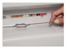
**Strapping** Manual bale strapping with Quick-link wire.
