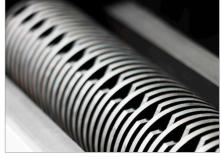
Specially hardened solid steel cutting rollers
