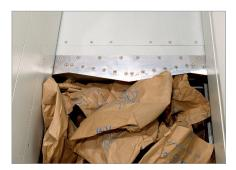
**Automatic operation** Control of the pressing process via light barrier.
