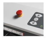
When the emergency stop switch is actuated, the device stops immediately.
