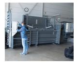
Safeguarding of the operating area with infrared light curtains for maximum operator safety
