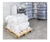
The lever action allows the HSM V-Press 60 to produce wellcompressed, stackable bales
