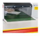
The material feeding is convenient and takes place via the non-slip conveyor belt.
