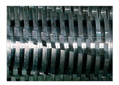
Specially hardened solid steel cutting rollers
