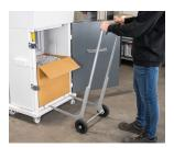
The removal trolley allows for the easy removal and disposal of the compact bales.
