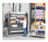
To fill the press, the upper half of the doors is pushed down and automatically opens after the compression process
