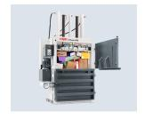
To fill the press, the upper half of the doors is swung to the right
