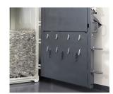
Double quantity of retaining claws optimize the compression of the pressing material and reduce the number of loading actions
