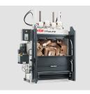
To fill the press, the upper half of the doors is pushed down and automatically opens after the compression process
