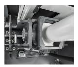
Gimballed press cylinder system -Reduced wear on the pressing cylinder and press ram guides
